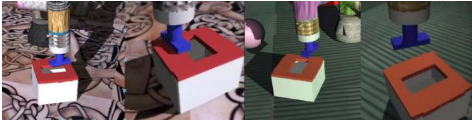
Figure 3.8: Examples of failure scenarios during the assembly phase where the trained model fails to insert the peg due to misalignment.
