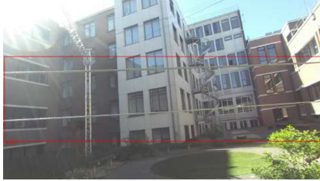
Figure 3.7: Detected power lines with the estimated distance (GT = 2 m)
