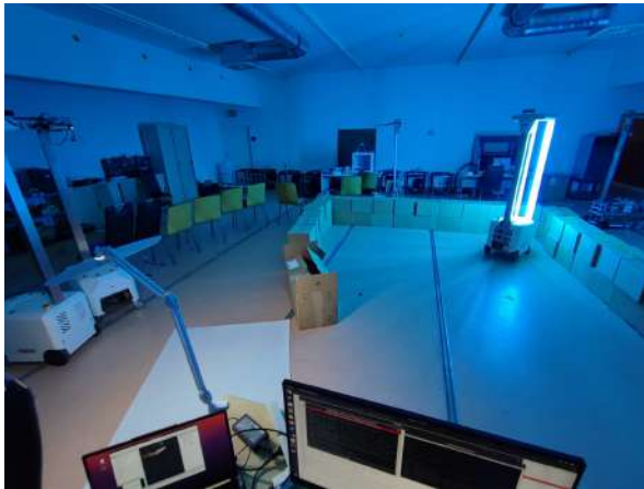
(a) Test Environment in No Overhead Light Scenario with the robot's UVC lights on.
