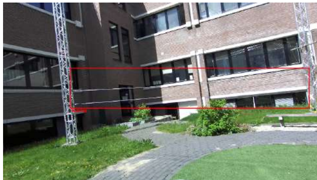
Figure 3.9: Detected power lines with the estimated distance (GT = 7 m)
