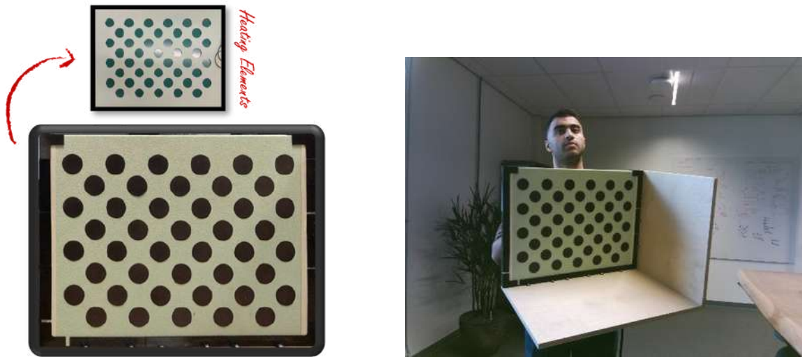
Figure 3.14: Custom circular grid calibration board with heating elements
