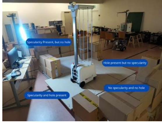
Figure 3.5: Test bench used to train and validate the SVM in the RT-SpecFilter
