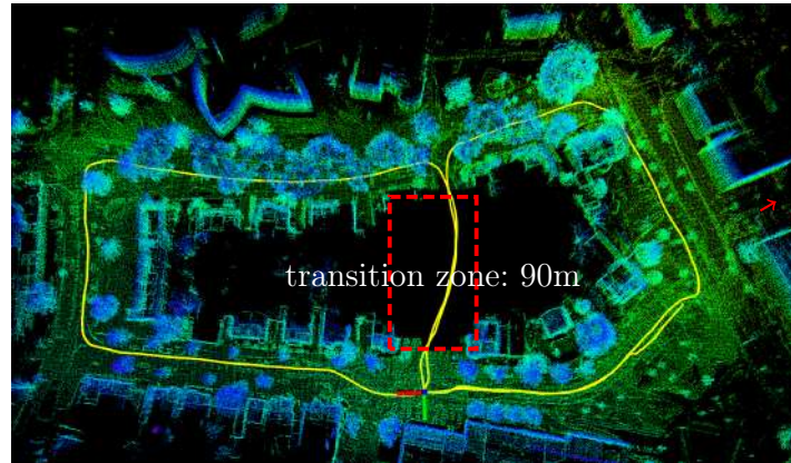
Figure 5.8: Localization in transition zone. The robot enters a transition region (highlighted in red) where LiDAR scan matching fails due to the absence of stable features in the prebuilt map
