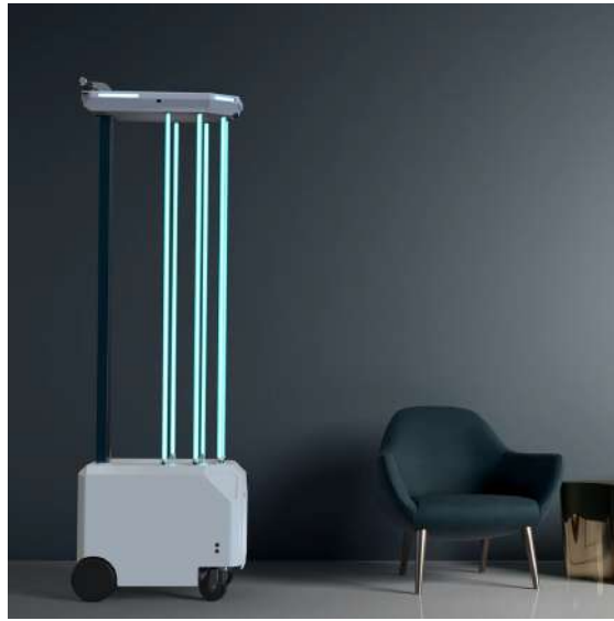
Figure 1.1: The Euroknows Virofighter, an autonomous UVC-light disinfection robot equipped with an Intel RealSense D435 RGB-D sensor and 4 wide field of view cameras
