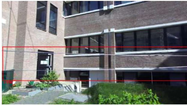
Figure 3.8: Detected power lines with the estimated distance (GT = 3.5 m)
