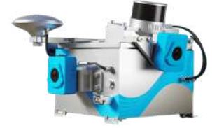
Figure 1: SDX-Compact, a versatile sensor rig for accurate outdoor surveying. It includes one Hesai Pandar XT32 LiDAR, one Septentrio INS with RTK, and three ArkCam RGB cameras.
