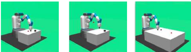
Fig 3: Experimental setup of Gymnasium Fetch benchmark tasks: FetchPush, FetchPickAndPlace, and FetchSlide.
